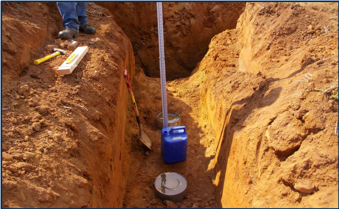
Photo 7.4 - Double Ring Infiltrometer Testing, Site A. Representative of both sites.
