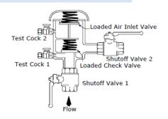
**Installation and testing requirements:** Commonly used in outdoor applications for protection in high or low hazard situations. Will not prevent backflow from backpressure, so it is required to be installed 12 inches above the highest downstream outlet (or above the highest point in the system). Annual testing required.
