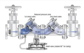
reduced pressure zone backflow preventer provides the highest level of protection.
