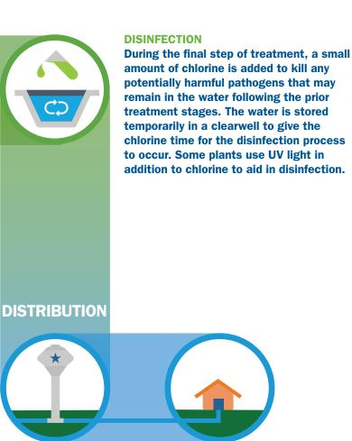
Pumps are typically used to "push" the water through pipes to homes and businesses in the community. Tanks are often used to provide storage around the distribution system to help maintain pressure and enhance reliability of water service and fire protection.
