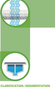
The heavy particles (floc) settle out and the clear water flows to filtration. The settled solids removed from the process often possess exceptional nutrient and water-retaining properties that allow them to be recycled and used to improve the quality of topsoils.
