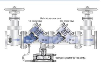
**Installation and testing requirements:** Due to certain combinations of check valve failure and/or system backpressure cause the relief valve to discharge, the device must be mounted in a location where the drain will not become flooded. Annual testing is required. This device can be installed either horizontally or vertical, per manufacturer recommendation.
