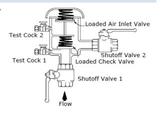
**Installation and testing requirements:** Commonly used in outdoor applications for protection in high or low hazard situations. Will not prevent backflow from backpressure, so it is required to be installed 12 inches above the highest downstream outlet (or above the highest point in the system). Annual testing required.
